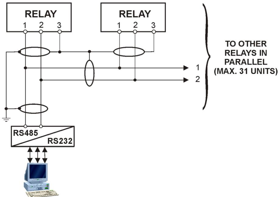
For longer distance and for connection of up to 250 Relays, optical interconnection is recommend. (please ask Microelettrica for accessories)
