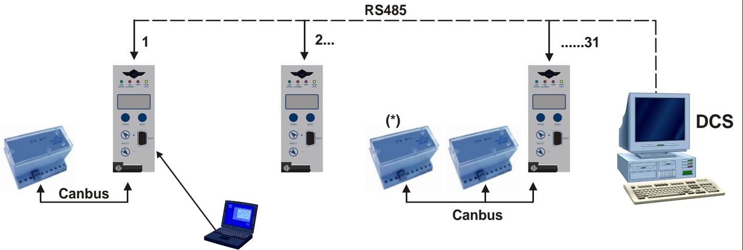
(\*) EX/IO - Expansion module = 5 Digital Inputs and 5 Relay Outputs
