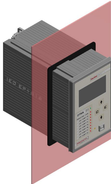
S16 semi-flush mounting method (max. depth = 75mm)
